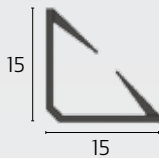
IS1515 perimeter seal – (15mm x 15mm) Retrofit self-adhesive seal with proven smoke & acoustic performance.
