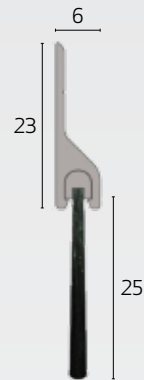
IS5120 brush seal – 25mm nylon brush seal mounted in an aluminium housing, screw fixed to the head and stiles of the steel angle surround.
